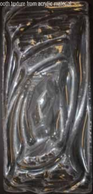
vaccum formed model smooth texture from acrylic material
